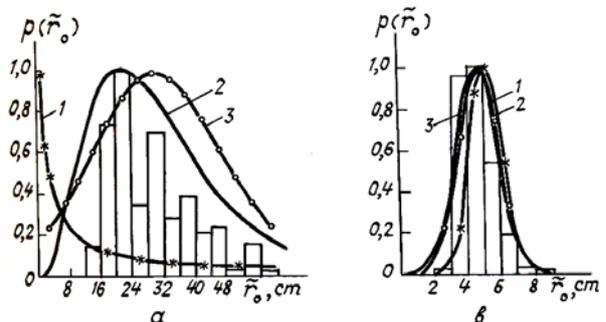
Fig. 2. Histograms of the probability distributions for  $\tilde{r}_0$ : a)  $D/r_0 = 3.75$ ; b)  $D/r_0 = 21$ ; 1) log-normal distribution; 2) gamma distribution; 3) normal distribution.
