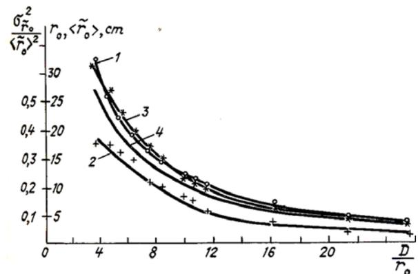
Fig. 1. Statistical characteristics of  $\tilde{r}_0$ : 1) mean value  $\langle \tilde{r}_0 \rangle$ ; 2) relative variance  $\sigma_{\tilde{r}_0}^2 / \langle \tilde{r}_0 \rangle$ ; 3)  $\langle \tilde{r}_0 \rangle$  determined by Eq. (5); 4) Fried parameter  $r_0$ .
