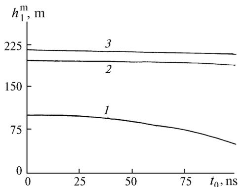
FIG. 3. Dependence of  $h_1^m$  on  $t_0$  at  $A = 10^{17} \text{ m}^2$ ,  $k_{lf} = 0.04$ ,  $\bar{B}_i = 0$ ,  $\varepsilon_1 = 0.15 \text{ m}^{-1}$ , and  $\varepsilon_2 = 0.125$  (1), 0.068 (2), 0.047  $\text{m}^{-1}$  (3).
