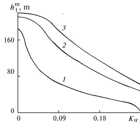
FIG. 4. Dependence of  $h_1^m$  on  $k_{lf}$  at  $A = 10^{17} \text{ m}^2$ ,  $t_0 = 0$ ,  $\varepsilon_1 = 0.15 \text{ m}^{-1}$ ,  $\bar{B}_i = 0$ , and  $\varepsilon_2 = 0.125$  (1), 0.068 (2), and 0.047  $\text{m}^{-1}$  (3).
