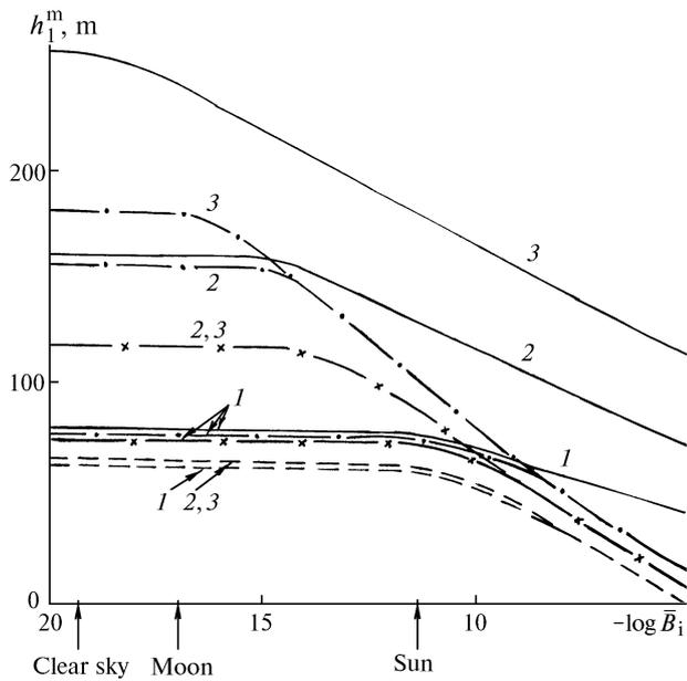
FIG. 5. Dependence of  $h_1^m$  on  $(-\log \bar{B}_i)$  at  $\epsilon_1 = 0.2 \text{ m}^{-1}$ ,  $\epsilon_2 = 0.08 \text{ m}^{-1}$ ,  $t_0 = 30 \text{ ns}$ , and  $A = 10^{10}$  (1),  $10^{15}$  (2), and  $10^{20} \text{ m}^2$  (3): —,  $k_{lf} = 0$ ; —·—, 0.04; —x—, 0.1; ----, 0.2.
