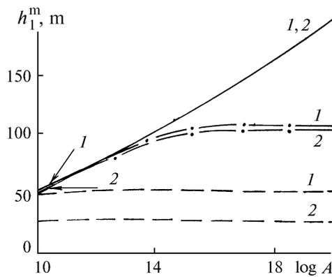
FIG. 2. Dependence of  $h_1^m$  on  $\log A$  at  $\varepsilon_1 = 0.3 \text{ m}^{-1}$ ,  $\bar{B}_i = 0$ ,  $t_0 = 0$  (1) and 50 ns (2), and  $k_{lf} = 0$  (solid curves), 0.01 (dot-and-dash curves), and 0.025 (dashed curves).
