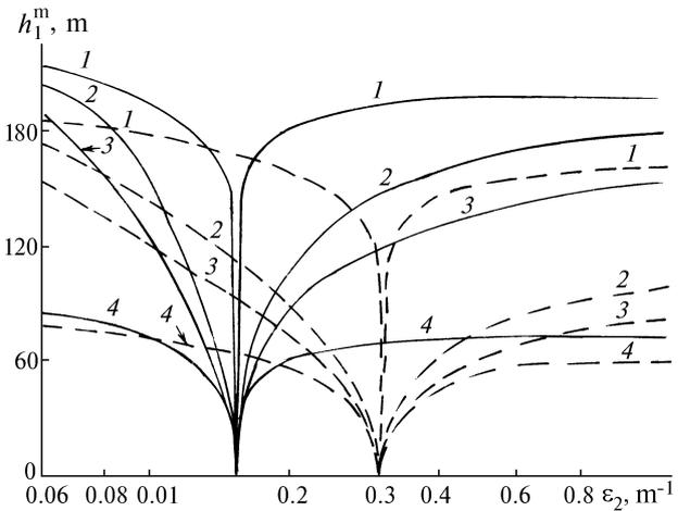
FIG. 1. Dependence of  $h_1^m$  on  $\varepsilon_2$  at  $\bar{B}_i = 0$  and  $\varepsilon_1 = 0.15$  (solid curves) and  $0.3 m^{-1}$  (dashed curves);  $k_{lf} = 0$  (1),  $0.04$  (2), and  $0.06$  (3 and 4);  $A = 10^{17}$  (1–3) and  $10^{10} m^2$  (4).
