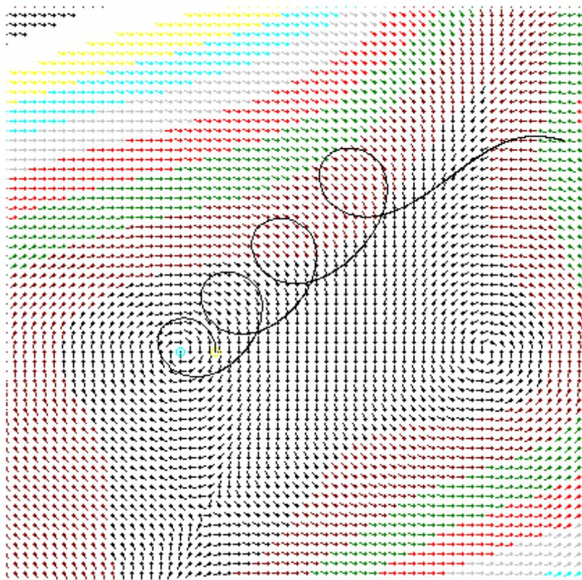
FIG. 1. The Poynting vector field on the plane perpendicular to the propagation axis (arrows) and the projection of spatial energy streamline on a given plane (solid line).
