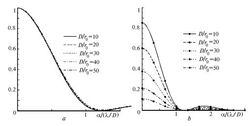
FIG. 4. AST-10 PSF, when the segmented adaptive mirror with 84 elements of hexagonal form is used. Every segment is controlled by the position and slopes. a - PSF is normalized by its axial value. b - PSF is normalized by the diffraction maximum.
