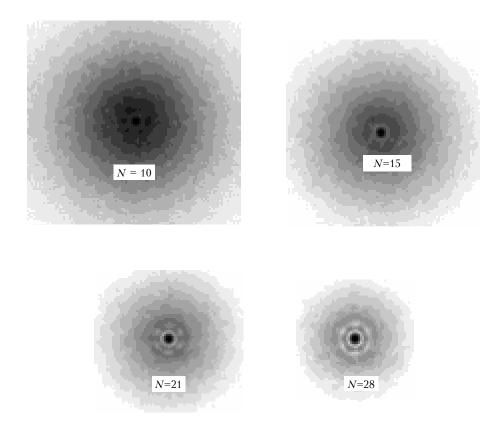
FIG. 1. Two-dimensional intensity distribution of AST-10 PSF for the modal compensation. Value of the aperture normalized diameter is  $D/r_0 = 20$ .
