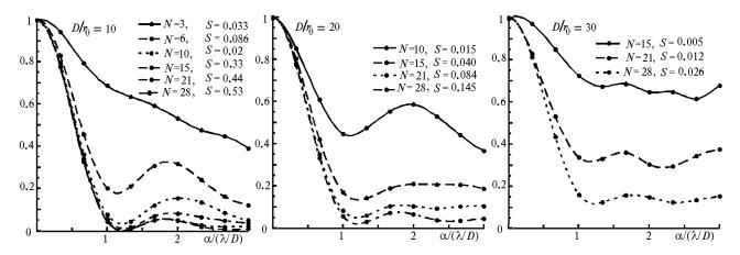
FIG. 2. AST-10 PSFs, when a modal corrector is used. Parameter N corresponds to the number of Zernike polynomials. PSF is normalized to the axial value. S is the Strehl ratio.
