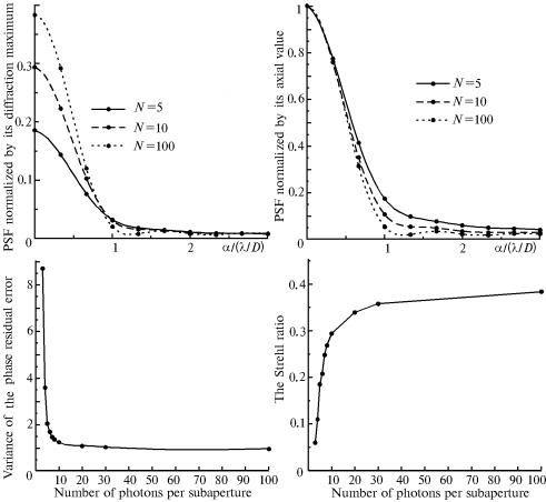
FIG. 6. Results of the simulation of an adaptive telescope with the Shack-Hartmann sensor. Normalized diameter of the aperture is  $D/r_0 = 10$ . Dimensions of the sensor lens diaphragm are  $10 \times 10$ . Estimation of the wavefront aberrations was performed by the modal algorithm (28 Zernike polynomials). Parameter N corresponds to the average-statistical number of photons at the subaperture during one exposure.
