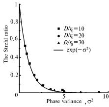
FIG. 3. The Strehl ratio as a function of the variance of phase residual distortions.
