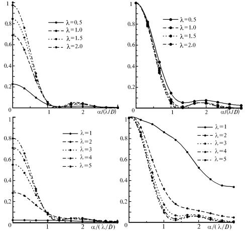
FIG. 7. PSFs of the AST-10 at different wavelengths for the adaptation using a laser reference star. Upper plots are for the sodium LRS (H = 100 km), the lower plots are for the Rayleigh LRS (H = 10 km). At the left plots the PSF is normalized to the diffraction maximum, at the right plots the PSF is normalized to its axial value. The wavelength  $\lambda$  is given in  $\mu$ m.
