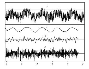
FIG. 2. Versions of the initial signal filtration: the initial curve (1); the result of processing of the initial curve by the low-pass filter with the cut-off frequency of 2 Hz (2); the result of processing of the initial curve by band-pass filter with the transmission frequency of 2–10 Hz (3); the result of processing of the initial curve by the high-pass filter with the cut-off frequency of 10 Hz (4).
