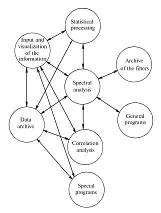
FIG. 1. Structural scheme of the software package "Random Signals Analyzer".
