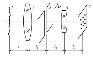
FIG. 1. Block diagram of the multichannel slit analyzer of a wave front of optical radiation.
