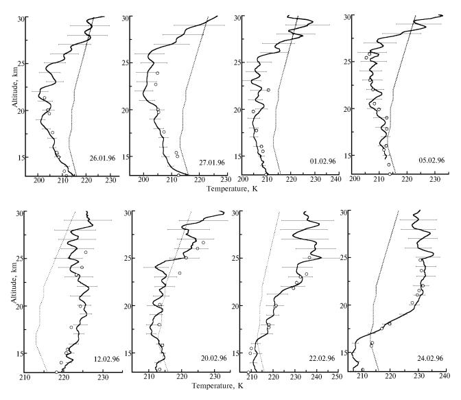
FIG. 1. Comparison of the results of temperature measurements with a lidar (solid curve), radiosondes (circles) for January-February of 1996, as well as the model profile (dotted curve).
