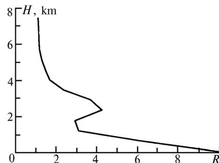
FIG. 4. Profile of the scattering ratio obtained when sounding the troposphere at a wavelength of 0.532  $\mu\text{m}$ .
