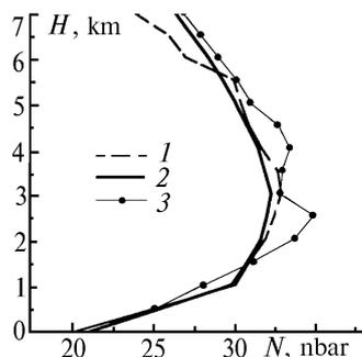
FIG. 5. Profiles of the tropospheric ozone concentration corrected for the aerosol contribution and derived from the data of multifrequency lidar at  $\lambda_{\text{on}} = 0.271 \mu\text{m}$  and  $\lambda_{\text{off}} = 0.289 \mu\text{m}$ : 1) profile obtained by the differentiation algorithm, 2) exact profile, and 3) profile obtained by the differential scheme.
