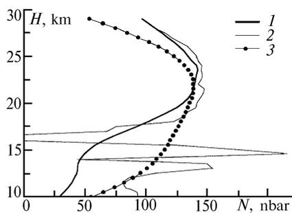
FIG. 1. Ozone concentration profiles obtained without their correction for aerosol contribution at  $\lambda_{on} = 0.308 \mu\text{m}$  and  $\lambda_{off} = 0.353 \mu\text{m}$ : 1) exact profile, 2) profile obtained by differential scheme, and 3) profile obtained by the algorithm of differentiation of empirical dependence.
