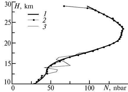
FIG. 3. Profiles of the stratospheric ozone concentration corrected for aerosol contribution and derived from the data of multifrequency lidar at  $\lambda_{\text{on}} = 0.308$   $\mu\text{m}$  and  $\lambda_{\text{off}} = 0.353$   $\mu\text{m}$ : 1) exact profile, 2) profile obtained by the regularization algorithm and 3) profile obtained by the differential scheme.
