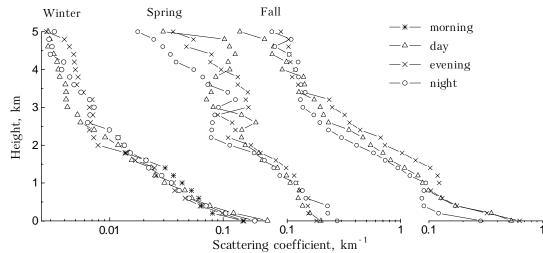
FIG. 1. Diurnal behavior of the vertical profile of the scattering coefficient of dry matter of aerosol particles in winter, spring and fall.
