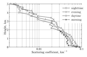
FIG. 3. Diurnal behavior of the vertical profile of the scattering coefficient of dry matter of aerosol particles in summer.
