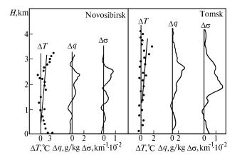
FIG. 5. Vertical profiles of changes in the scattering coefficient, temperature and specific humidity occurring during the time between two cycles of sounding during a summer day under anticyclonic conditions.
