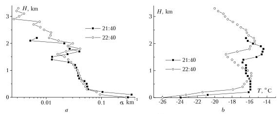
FIG. 2. Vertical profiles of aerosol scattering coefficient (a) and temperature (b) measured on January 14, 1986, over the town of Kolpashevo with the time interval of 1 hour.
