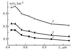
FIG. 2. Spectral structure of aerosol extinction coefficients in rural haze at relative humidity R = 63 (curve 1), 80 (curve 2), and 96 per cent (curve 3).
