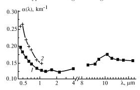
FIG. 1. Spectral structure of aerosol extinction coefficients under conditions of urban (1) and rural (2) hazes.
