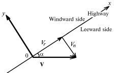
FIG. 1. Geometrical relationships between the wind and road directions: V is the wind vector,  $V_n$  and  $V_r$  are the projections of the wind vector to the road direction (x) and to the direction normal to it (y-axis);  $\alpha$  is the angle between the road and the wind vector directions.
