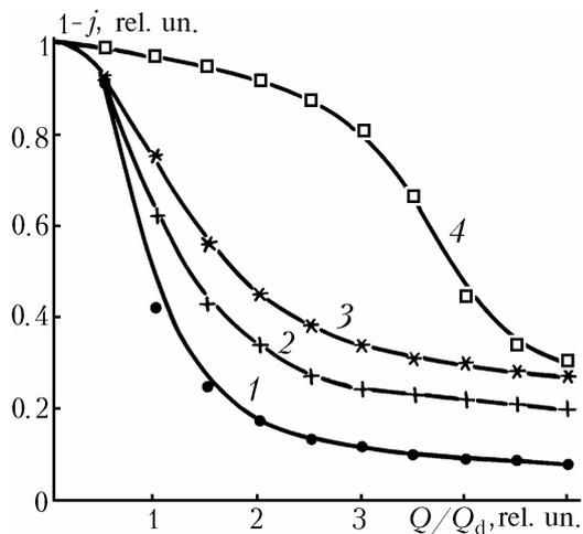
FIG. 3. Angular distribution of the pump beam energy passed through the cold cell (1), the cell with metal vapor at  $T = 850$  (2) and  $1300^\circ\text{C}$  (3) as well as the SRS radiation (4);  $j$  denotes the portion of the radiation energy within the corresponding angle  $Q$  with respect to the total energy,  $Q_d$  denotes the diffraction angle.
