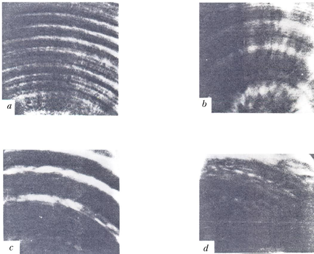
FIG. 2. Fragments of interferograms of the pump beam with the linewidth of 0.01 (a) and 0.1 cm<sup>-1</sup> (b) and the corresponding SRS radiation (c and d). The etalon free dispersion region was 0.07 (a) and 0.25 cm<sup>-1</sup> (b, c, and d).
