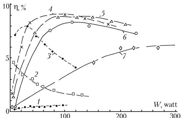
FIG. 1. Efficiency of XeCl\* radiation versus pumping power, Xe:Cl<sub>2</sub> = 3:1 gas mixture at the total pressure < 0.25, 0.25, 0.5, 1, 2, 4, and 6 Torr.
