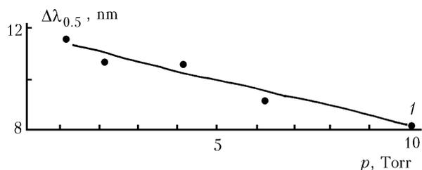
FIG. 2. Bandwidth (FWHM) of spontaneous radiation of XeCl\* molecules versus total pressure of Xe:Cl<sub>2</sub> = 3:1. Point 1 was obtained in Xe:HCl = 3:1 gas mixture.
