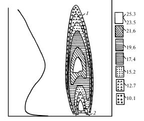
FIG. 1. Thermogram of the stationary discharge 1 formed by the pointed electrode 2.
