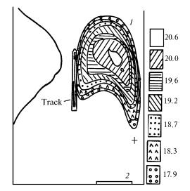
FIG. 5. Thermogram of the transient regime with the particle track shown to the left: discharge 1 and electrode 2.
