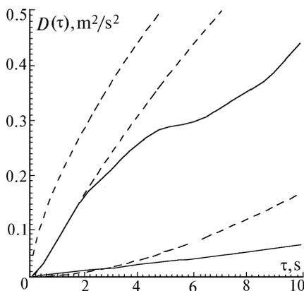
FIG. 5. Structure functions of the wind velocity measured with the Doppler lidar at  $\Delta z = 2.3$  (1, 1') and 62 m (2, 2'); experiment (1, 2); theory (1', 2'); the structure function from point measurements of the wind velocity (1').
