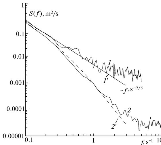
FIG. 3. Wind velocity spectra measured with an acoustic anemometer (1, 1') and a Doppler lidar (2, 2'); experiment (1, 2); theory (1', 2').
