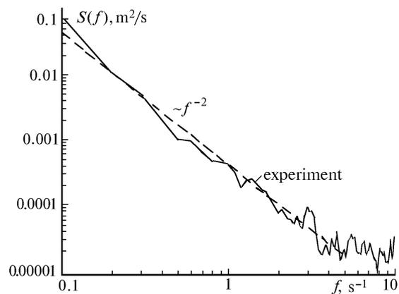
FIG. 6. The wind velocity spectrum measured using a Doppler lidar for a large sounding volume ( $\Delta z = 260$  m) with the wind direction along the beam axis.
