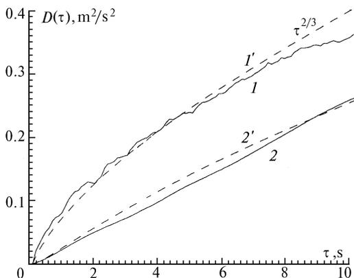
FIG. 2. Structure functions of the wind velocity measured with an acoustic anemometer (1, 1') and a Doppler lidar (2, 2'); experiment (1, 2), theory (1', 2').
