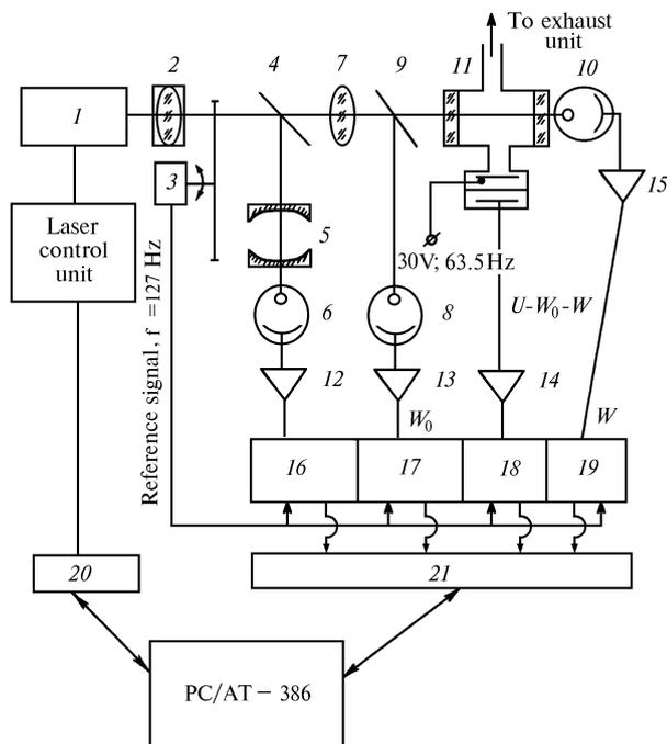
FIG. 1. Block diagram of the combined diode laser spectrometer.
