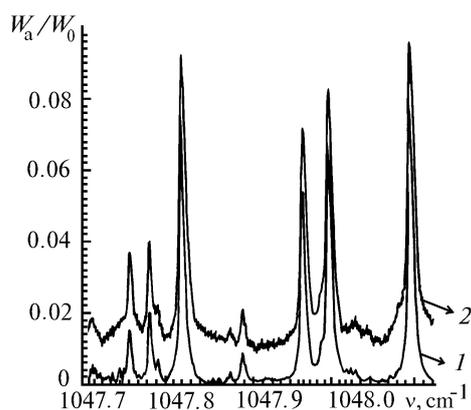
FIG. 2. The absorption spectrum of ozone in argon measured by the spectrophotometric (1) and photoacoustic (2) methods;  $W_0$  is the power at the cell input,  $W_a$  is the power absorbed in the cell.
