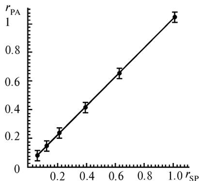
FIG. 3. Comparison of the measurement results for the absorption coefficient at the line center at different pressures of ozone obtained by the spectrophotometric ( $r_{SP}$ ) and photoacoustic ( $r_{PA}$ ) methods.
