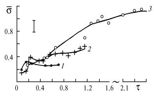
FIG. 1. Average values of fluctuation level  $\sigma$  vs optical depth  $\tau$  for D = 3.1 mm:  $D_{\rm m} = 1 \text{ mm}(1)$ , 1–3 mm(2), and 5 – 10 mm(3).
