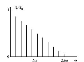
FIG. 1. The spectrum of the narrow-band noise envelope at the output of narrow-band system with  $\Pi$ -shaped AFC.
