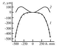
FIG. 1. Correction planoid profile of the Schmidt system: 1) profile of the corrector located in the center of a spherical mirror; 2) profile of the corrector displaced at a distance of 7.5 mm.
