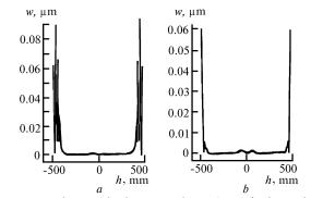
FIG. 2. The residual wave aberration of the Schmidt system for the correctors shown in Fig. 1: a) profile 1 and b) profile 2.
