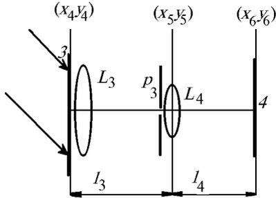
FIG 2. The optical scheme of recording the interferogram located in the hologram plane.
