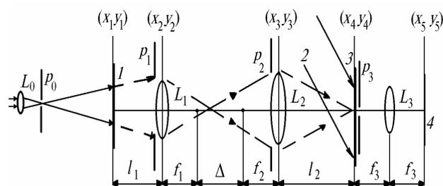
FIG 1. The optical scheme used for recording and reconstruction of double-exposure Fourier hologram: mat screen (1), reference beam (2), photographic plate - hologram (3), interferogram plane (4), lenses *L*<sub>0</sub>, *L*<sub>1</sub>, *L*<sub>2</sub>, *L*<sub>3</sub>, filtering diaphragms *p*<sub>0</sub> and *p*<sub>3</sub> and aperture diaphragms *p*<sub>1</sub> and *p*<sub>2</sub>.
