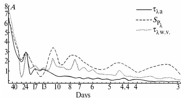
FIG. 3. Amplitude spectrum of oscillations of the spectral transmission ( $S_{p\lambda}$ ), aerosol optical thickness ( $\tau_{\lambda a}$ ), and total content of water vapor ( $\tau_{\lambda w.v.}$ ).
