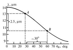
FIG. 1. Radiation wavelength at the exit from a wedgeshaped interference filter as a function of the refraction angle  $\sigma_n$  (n = 3, l = 1 mm).
