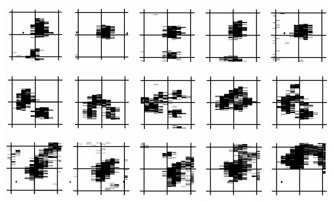
FIG. 9. Vertical sections of electric-power-station smoke plume vs. time (time interval of 2 min) and distance from stack mouth of 50 (upper row), 100 (middle row), and 150 m (lower row). The size of map grid is 75×75 m.
