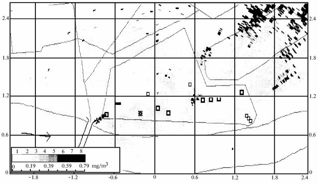
FIG. 8. Mapping of aerosol pollution distribution in azimuth scanning at angle of 10° at Kemerovo. The location of lidar is marked as 0 on the ordinate.
