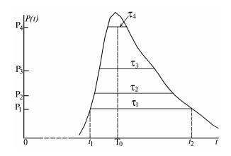
FIG. 13. The diagram of return record by a satellite laser range finder with four threshold layers.
