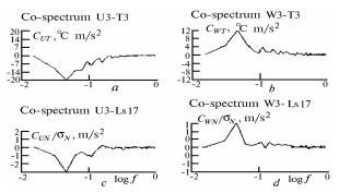
FIG. 4. Co-spectra of horizontal heat flows (a) and aerosol content (c), and the corresponding vertical flows of these quantities (b and d).
