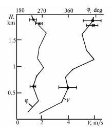
FIG. 12. The profiles of wind velocity and direction in drizzle, as measured by three-path lidar. The horizontal bars show the confidence interval at a probability of 0.95.
