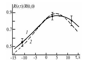
FIG. 7. The experimental (1) and theoretical (2) correlation functions of returns at 2.5 m altitude. Vertical bars show rms deviations.
