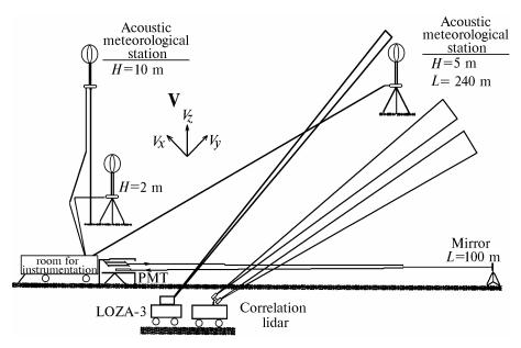
FIG. 1. Scheme of the laser-acoustic experiment to study atmospheric aerosol.
