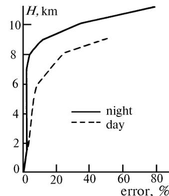
FIG. 3. Results of numerical simulation of the error of water vapor sounding from RS signals.
