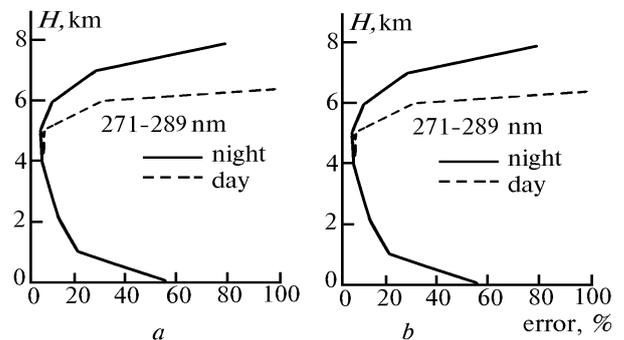
FIG. 2. Results of numerical simulation of ozone sounding error at wavelengths of 271–289 nm (a) and 289–308 nm (b).
