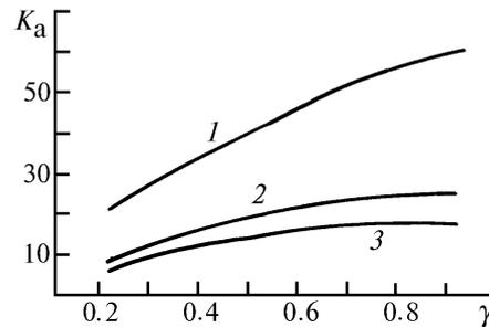
FIG. 4. The dependence  $K_a = f(\gamma)$  for a single additional dosage capacitor:  $\alpha = 0.01$  (1), 0.05 (2), and 0.1 (3)
