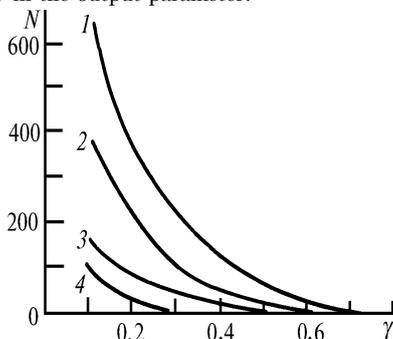
FIG. 2. The function  $N = f(\gamma)$  for different relative uncertainties in output parameter:  $\alpha = 0.01$  (1),  $0.02$  (2),  $0.05$  (3), and  $0.1$  (4)
