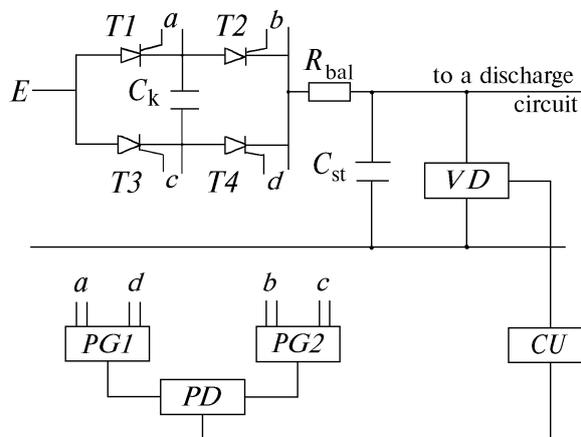
FIG. 1. Block-diagram of a charging device with a dosage capacitor: a voltage divider (VD), control unit (CU), pulse distributor (PD), and pulse generators (PG1 and PG2), which triggers the thyristors  $T1$  and  $T4$  and  $T2$  and  $T3$ , respectively
