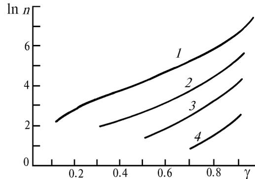
FIG. 3. The function  $n = f(\gamma)$  for relative uncertainty in output parameter  $\alpha = 0.1$  at various values of lower limit of regulation:  $\gamma_{low} = 0.1$  (1),  $0.3$  (2),  $0.5$  (3), and  $0.7$  (4)
