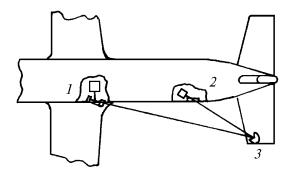
Fig. 1. Layout of instrumentation placed on board the aircraft.
