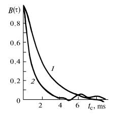
FIG. 4. Normalized autocorrelation function for the scattered radiation at  $\varphi = 0.5$  mrad: 1)  $D_{\rm M} = 10-20$  mm,  $\sigma^2 = 1.03$ ,  $\tau = 0.2$ , V = 2 m/s, and V = 1.8 m/s; 2)  $D_{\rm M} = 1-2$  mm,  $\sigma^2 = 0.55$ ,  $\tau = 0.3$ , V = 3.4 m/s, and V = 1.2 m/s.
