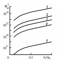
FIG. 3. The variance of the phase fluctuations reconstructed over the beam cross section.  $\Delta z = 10^{-4}$  (1),  $3 \cdot 10^{-4}$  (2),  $5 \cdot 10^{-4}$  (3),  $10^{-3}$  (1), and  $10^{-2}$  m (5).
