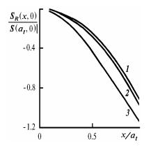
FIG. 1. The general view of the reconstructed mean phase of a single-mode Gaussian beam for different longitudinal bases of measurements  $\Delta z$ : 1) exact values of the phase for  $\Delta z = 10^{-4}$ ,  $3 \cdot 10^{-4}$ ,  $5 \cdot 10^{-4}$ ,  $10^{-3}$ ,  $10^{-2}$  m; 2)  $\Delta z = 10^{-1}$  m; and, 3)  $\Delta z = 5 \cdot 10^{-1}$  m,  $\gamma = 5$ .
