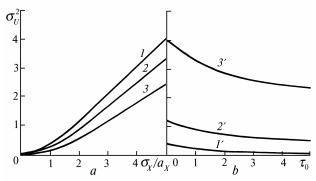
FIG. 3. The relative variance  $\sigma_U^2$  as a function of the ratio  $\sigma_{x'}/a_x$  (a) and optical thickness of a plume  $\tau_0$  (b): 1)  $\tau_0 = 0.1$ ; 2)  $\tau_0 = 1$ ; 3)  $\tau_0 = 5$ ; 1')  $\sigma_{x'}/a_x = 1$ ; 2')  $\sigma_{x'}/a_x = 2$ ; 3')  $\sigma_{x'}/a_x = 5$ .
