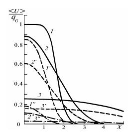
FIG. 1. Mean intensity distribution: 1, 1', and 1")  $\sigma_x/a_x=0$ ; 2, 2', and 2")  $\sigma_x/a_x=1$ ; 3, 3', and 3")  $\sigma_x/a_x=5$ ; 1, 2, and 3)  $\tau_0=5$ ; 1', 2', and 3')  $\tau_0=1$ ; and 1", 2", and 3")  $\tau_0=0.1$ .
