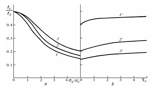
FIG. 4. The integral scale of intensity fluctuations correlation as a function of  $\sigma_{\chi}/a_x$  (a) and  $\tau_0$  (b): 1)  $\tau_0 = 0.1$ , 2)  $\tau_0 = 1$ , 3)  $\tau_0 = 5$ , 1')  $\sigma_{\chi}/a_x = 1$ , 2')  $\sigma_{\chi}/a_x = 3$ , and 3')  $\sigma_{\chi}/a_x = 5$ .
