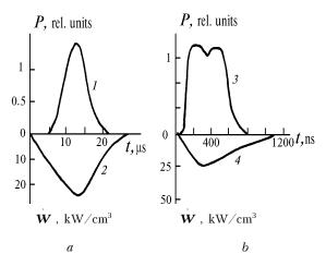
FIG. 1. Losing pulse waveforms at  $\lambda = 585.3$  nm (1) and (3) and the temporal dependence of excitation power (2) and (4) for the mixtures He : Ne : Ar = 1.0 : 0.27 : 0.02 atm (a) and He : Ne : Ar = 2.1 : 0.34 : 0.06 atm (b).
