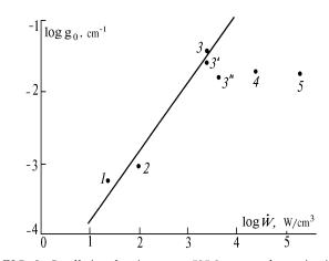
FIG. 2. Small-signal gain at  $\lambda = 585.3$  nm vs the excitation power. The numbers of close circles correspond to the line numbers in the table (see the text of this paper).
