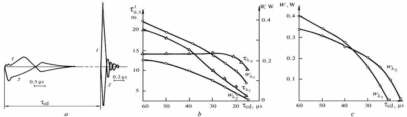
FIG. 3. Typical waveforms of current (1) and voltage (2) of the control pulses (on the left) and excitation pulses (on the right) (a). Dependence of the duration and average output power (b, c) for the green (1) and yellow (2) spectral lines on the time delay  $\tau_{cd}$ .
