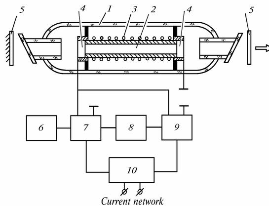
FIG. 4. Schematic diagram of a stabilized laser with a built-in resistance heater: 1) hermetically sealed case, 2) gas–discharge channel, 3) heater, 4) electrodes, 5) resonator mirrors, 6) pulse driver, 7) heating source, 8) timing unit, 9) excitation source, and 10) control unit.
