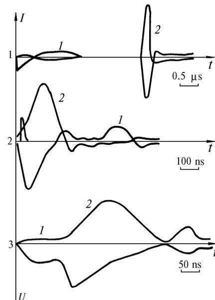
FIG. 6. Wave forms of the AP (1) and the EP (2) for different time delay: (a) the AP controls the output power and chromaticity through variations of  $n_e$  and  $N_m$ , (b) the AP is used as an additional heater, and (c) superposition of the AP and the EP results in a “complex” shape of the pumping current pulse with long risetime.
