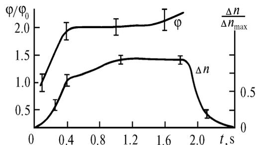
FIG. 2. A comparison between the angular size of the HPR beam at the far end of the path and variation in  $\Delta n$  inside the active channel.
