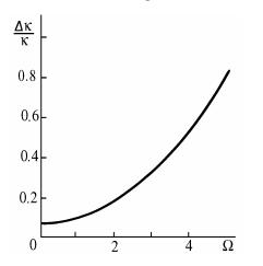
FIG. 2. Dependence of relative error in measurements of the absorption coefficient on the frequency detuning from an absorption line center.
