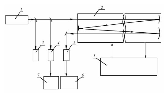
FIG. 1. Block diagram of the laser spectrophotometer: 1) laser, 2) multipass gas absorption cell, 3) wavelength meter, 4 and 5) photodetectors, 6 and 7) digital voltmeters, and 8) system for preparing and control of gas mixtures.
