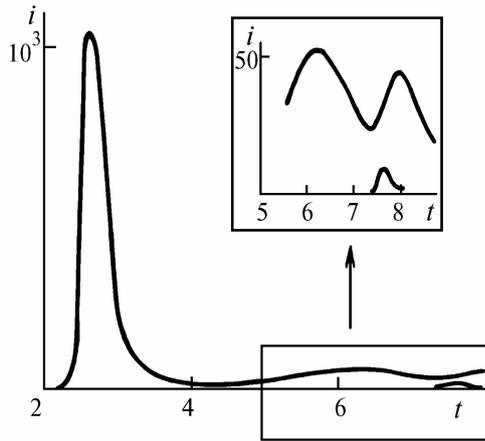
FIG. 1. Pulse shape of the hybrid  $\text{CO}_2$  laser at the echo-signal reception. The time scale is marked every 400 ns. The intensity is in relative units. For scale comparison the echo signal is shown separately above the curve of the pulse shape.
