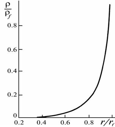
FIG. 2. Density distribution of combustion gases of propellant behind the shock wave front.
