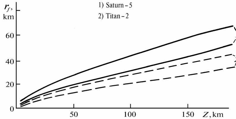
FIG. 3. Characteristic size of the jet flame  $r_f(z)$  in a segment of the trace typical of the nonautomodel regime at  $v_{\text{roc}} = 3$  (solid line) and 5 km/s (dashed line).
