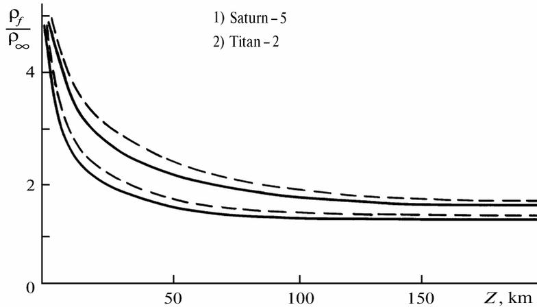
FIG. 4. Densities of particle condensation along the rocket flame axis at an altitude of 150 km at  $v_{\text{roc}} = 3$  (solid line) and 5 km/s (dashed line).
