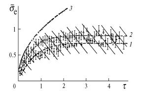
FIG. 1. Fluctuation level  $\sigma_{\rm e}$  averaged over all paths at different  $\tau$  for three values of the maximum diameter of snowflakes  $D_{\rm m}$ : 1)1-3, 2)3-5, and 3)7 mm on 650-m path.
