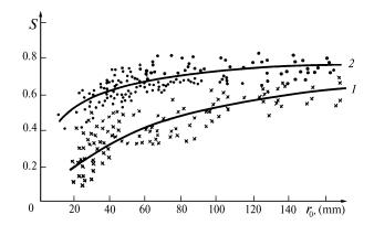
FIG. 1. Experimental results of correcting for atmospheric turbulence along a horizontal optical path. Curve 1 is for open–looped contour and curve 2 is for close–looped contour.
