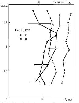
FIG. 2. Profiles of the wind speed V and direction W measured by the lidar and METEOR station on June 19, 1991. Horizontal bars indicate the 0.9 confidence level.
