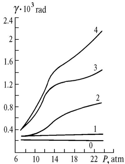
FIG. 3. Dependence of the divergence of the SRS conversion components of the XeCl laser on the pressure of hydrogen:  $\lambda = 308$  (0), 353 (1), 413 (2), 499 (3), and 628 nm (4).
