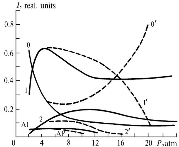
FIG. 4. Dependence of the intensity of components of the SRS conversion on the pressure: in pure hydrogen (A1, 0, 1, and 2), in hydrogen under initial pressure of 4 atm with subsequent addition of argon ( $A1'$ ,  $0'$ ,  $1'$ , and  $2'$ ).  $\lambda = 532$  (0), 683 (1), 954 (2), and 436 (A1) nm.
