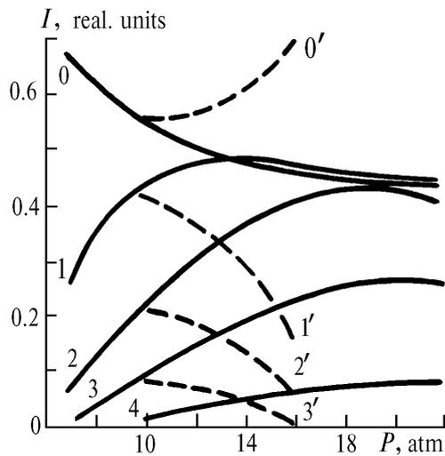
FIG. 2. Dependence of the intensity of components of the SRS conversion on the pressure: in pure hydrogen (0, 1, 2, 3, and 4); in hydrogen under initial pressure of 10 atm ( $0'$ ,  $1'$ ,  $2'$ , and  $3'$ ) with subsequent addition of argon.  $\lambda = 308$  (0), 353 (1), 413 (2), 499 (3), and 628 nm (4).
