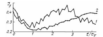
FIG. 3. Dynamic control of the beam phase based on the simplex method for two values of the simplex edge length: L = 0.6 (curve 1) and 0.3 (curve 2). Parameters of propagation:  $z_0 = 0.5$  and R = -20.
