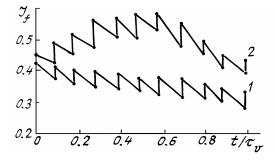
FIG. 4. Beam phase control for "frozen" instantaneous states of the medium ( $\tau_c = 0.01\tau_v$ ). 1) L = 0.1 and 2) L = 0.2. Parameters of propagation:  $z_0 = 0.5$  and R = -20.
