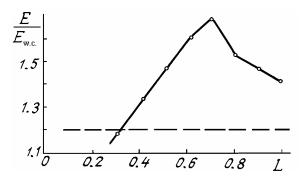
FIG. 2. The total relative light energy  $E/E_{wc}$  falling within the receiving aperture during the control time  $T = 3\tau_r$  as a function of the simplex edge length L (dashed line is for the gradient method with an optimal step). Parameters of propagation:  $z_0 = 0.5$  and R = -20.  $E_{wc}$  is the energy in the system without control.
