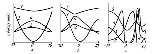
FIG. 2. The time dependences of the lasing power (1), the difference between the populations of the working levels of the active medium (2), and the populations of the lower (3) and upper (4) levels of the absorbing medium: a)  $\varepsilon = 0$ ; b)  $\varepsilon = 5 \cdot 10^{-3}$ ; c)  $\varepsilon = 2 \cdot 10^{-2}$ . The rest of the parameters are the same as in Fig. 1.
