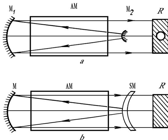
FIG. 1. The optical scheme of the XeCl laser with unstable telescopic resonators in which the output beam passed by the convex mirror  $M_2$  (a) through the partially reflecting specular meniscus SM (b):  $M$  and  $M_1$  are the concave mirrors of the resonator; AM is the active medium; and R is the output cross section of the laser beam.
