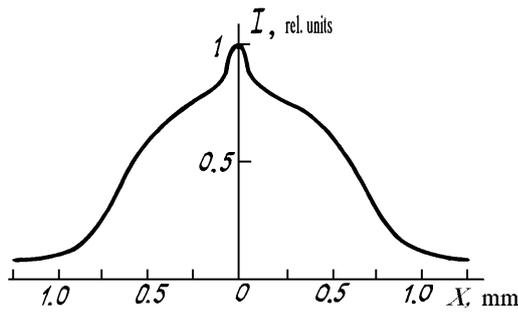
FIG. 2. The opacity density record of the focal spot of the laser beam formed by the concave mirror—specular meniscus resonator with  $\rho_{SM} = 20\%$  at  $M = 10$ . The focal length of the lens  $F = 32.4$  cm.
