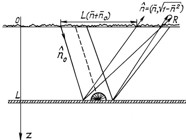
FIG. 2. Reflection of the paraxial beam from the layer of the diffuse scatterers in the homogeneous medium: Unperturbed problem.
