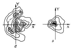
FIG. 4. Intensity isophotes in the beam crosssection (far zone of diffraction) for  $|R_{o}| = 640$ . a) in the "off" mode of control; b) in the "on" mode of control. The origin of the coordinate system coincides with the beam energy center  $(z_{c}, y_{c})$ . Dashed curve shows the receiving aperture.
