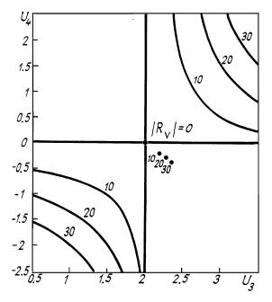
FIG. 1. Coordinates of the minimum of functional of focusing  $\hat{F}_3$  and curves of zero functional of astigmatism  $\hat{F}_4$  in the plane of modal control  $(U_3, U_4)$  for different values of the nonlinearity parameter  $R_{\gamma}$ . Path length  $z = 0.5\kappa a_0^2$ .
