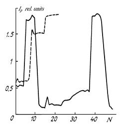
FIG. 2. Variation of the peak intensity of the beam  $I_p$  in the process of control by multicriterional algorithm (solid line) and by method of gradient optimization against a single
