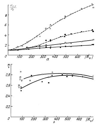
FIG. 3. Effective beam size  $a_x$  (filled squares and circles) and  $a_y$  (empty squares and circles); squares: v = 1.1 mm/s; circles: v = 2 mm/s; triangles: v = 3 mm/s. Dashed lines: in the "off" mode of control; Solid lines: in the "on" mode of control. a) effective size is. nonlinearity parameter  $R_v$ . b) control efficiency  $\eta$  is. nonlinearity parameter  $R_v$ .
