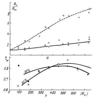
FIG. 6. Energetic radius of the beam  $a_W$ . a) Energetic radius  $a_W$  at 63% level of the total power vs  $R_v$ . Empty circles and crosses: flow speed v = 2 mm/s; squares; v = 1.1 mm/s; dashed lines: without control; solid lines: after control. Clear circles and squares: digitized image; crosses; PM data. b) Energetic efficiency of control  $\eta_W$  vs the parameter of nonlinearity  $R_t$  at 63% and 30% levels of the total power and for the flow speed t = 2 mm/s.
