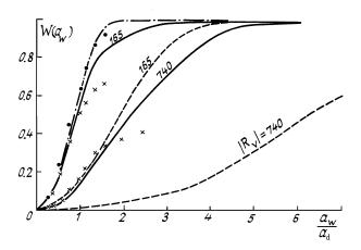
FIG. 5. Normalized power  $W(a_W)$  vs. receiving aperture radius  $a_W$ .  $a_d$  is the diffraction radius of a Gaussian beam. Data are obtained from the digitized image: dash-dot line shows the linear case  $R_0 = 0$ , dashed line shows the "off" mode of control; solid line shows the "on" mode of control. The PM data: dots indicate the linear case and crosses show the corresponding parameter after the control.
