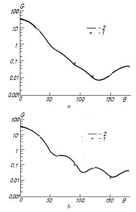
FIG. 1. Angular dependence of the values  $G_1(\theta)$  (a), and  $G_2(\theta)$  (b): 1) analytical calculations, and 2) calculations by formulas (10).
