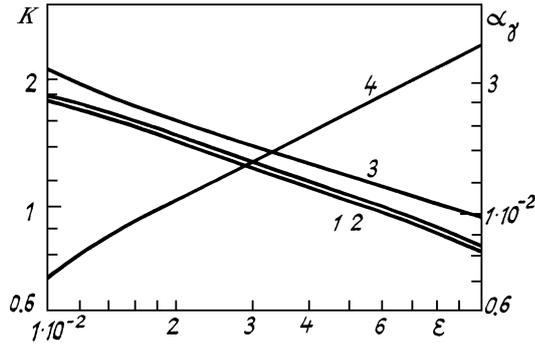
FIG. 1. Actual conditionality of the model inverse problem after regularization (curves 1–3), and the regularization parameter (curve 4) vs the error in the initial data.
