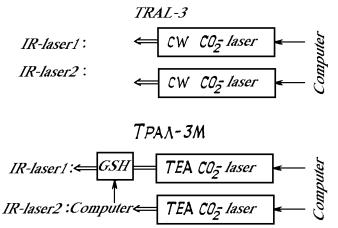
FIG. 2. Tunable IR molecular lasers for the "TRAL-3" and "TRAL-3M" models
