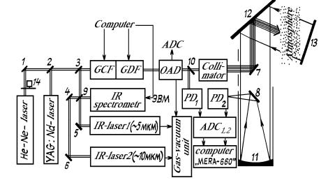
FIG. 1. Block diagram of the LGADA: movable mirrors (1–8), semi-transparent plates (9, 10), receiving mirror 30 cm in diameter (11), mirror-scanner (12), specular reflector (13) (in the case of "TRAL-3M" an option is possible with topographic target), and modulator (14).
