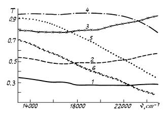
FIG. 3. Transmission spectrum (experiment) of the BS-4 glass particles dispersed in immersion liquids with  $n_D = 1.49$  (1), 1.50 (2), 1.51 (3), 1.52 (4), 1.53 (5), and 1.54 (6).
