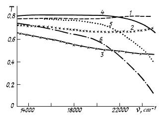
FIG. 6. Transmission of the layer of suspension of the BS-4 glass particles of radius 1 mm dispersed in immersion liquid with n = 1.49 (1), 1.52 (2), 1.51 (3), 1.52 (4), 1.53 (5), 1.54 (6). The thickness of the layer was 1 mm. Dots denote the results of calculations.
