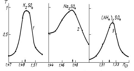
FIG. 2. Experimental curves of the transmission of the layer of suspension (d = 5 mm) as functions of the refractive index of immersion liquid: 1)  $K_2SO_4$ ; 2)  $Na_2SO_4$ ; 3)  $(NH_4)_2SO_4$ .
