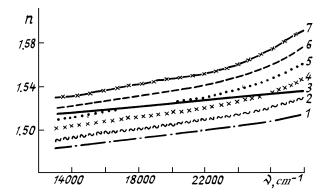
FIG. 1. Dispersion of the refractive indexes of the BS-4 glass (curve 1) and immersion liquids with  $n_D = 1.49$  (2), 1.50 (3), 1.51 (4), 1.52 (5), 1.53 (6), and 1.54 (7).
