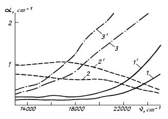
FIG. 4. Extinction coefficients of the layer of suspension of the BS-4 glass particles. The thickness of the layer was equal to 0. 1 and 1 cm.  $n_D = 1.52$  (1 and 1'), 1.51 (2 and 2'), 1.53 (3 and 3'), 1, 2, 3) d = 0.1 cm; 1', 2', 3') d = 1 cm.
