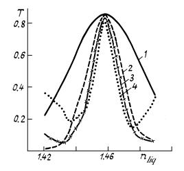
FIG. 5. Transmission of the layer of suspension of particles dispersed in immersion liquids (v = 1700 cm, d = 5 mm) for the particles with radii a = 1 (1), 5 (2), 10 (3), and 15 (4) mm. Dots denote the results of calculations.
