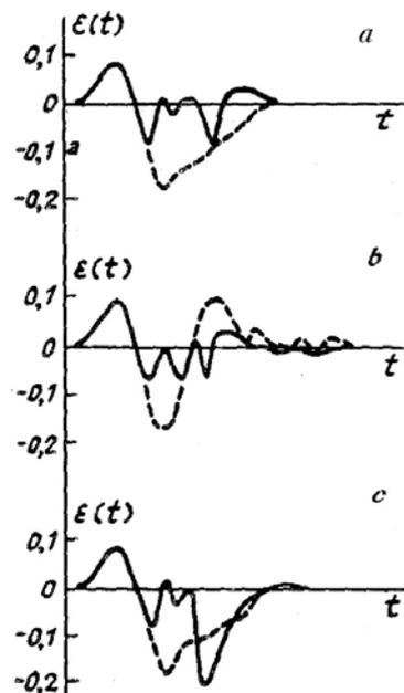
FIG. 2. Dependence of the optical pulse shape on the direction of propagation: the solid curve plots the results for downward propagation and the dashed curve — for upward propagation for  $q = 4$ ,  $\tau_p = 30 \text{ cm}$ , and  $\Delta = 0.1$  (a), 0 (b), and  $-0.1$  (c)  $\text{cm}^{-1}$ .
