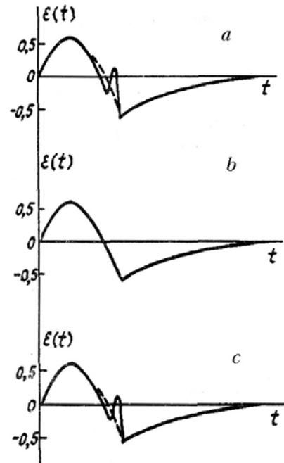
FIG. 4. Deformation of pulse shape in a resonantly absorbing atmosphere: the solid curve shows downward propagation and the dashed curve — upward propagation for  $q = 1$ ,  $\tau_p = 3 \text{ cm}$ , and  $\Delta = 0.1$  (a), 0 (b), and  $-0.1$  (c)  $\text{cm}^{-1}$ .
