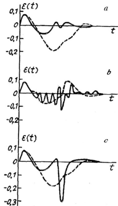
FIG. 1. Dependence of the optical pulse shape on the direction of propagation: the solid curve plots the results for downward propagation and the dashed curve — for the upward propagation for  $q = 1$ ,  $\tau_p = 30 \text{ cm}$ , and  $\Delta = 0.1$  (a), 0 (b), and  $-0.1$  (c)  $\text{cm}^{-1}$ .
