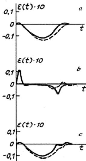
FIG. 3. Deformation of pulse shape in a resonantly absorbing atmosphere: the solid curve shows downward propagation and the dashed curve — upward propagation for  $q = 1$ ,  $\tau_p = 100 \text{ cm}$ , and  $\Delta = 0.1$  (a), 0 (b), and  $-0.1$  (c)  $\text{cm}^{-1}$ .
