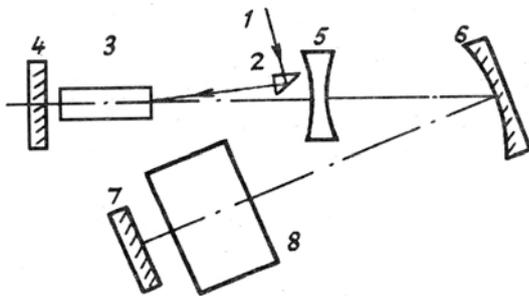
FIG. 1. Optical diagram of the laser. 1) pump radiation, 2) rotating prism, 3) active element, 4) output mirror, 5) negative lens, 6) spherical mirror, 7) nontransmitting mirror, and 8) selector.
