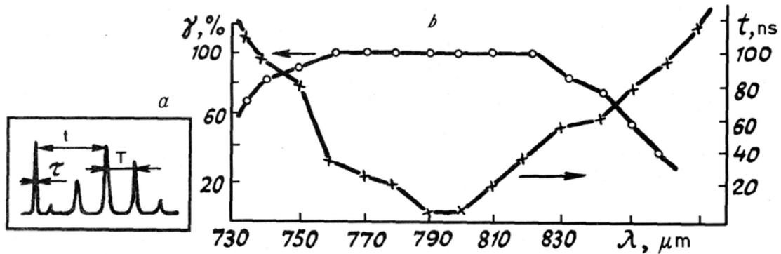
FIG. 2. Typical lasing time sweep in the HRRPT regime (a) and the degree of modulation  $\gamma$  and delay time  $t$  of the HRRPT relative to the maximum of the seed pulse (b).
